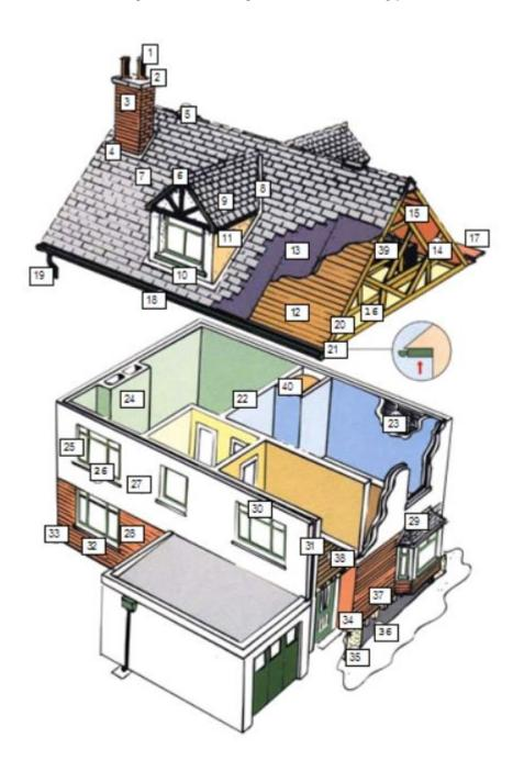
Dormer flashing 10 Dormer cheeks 11 12 Sarking Roof felt 13 Trusses 14 15 Collar 16 Insulation 17 Parapet gutter Eaves guttering 18 Rainwater downpipe 19 20 Verge boards / skews 21 Soffit boards 22 Partition wall Lath / plaster 23 24 Chimney breast 25 Window pointing Window sills 26 Rendering 27 Brickwork / pointing 28 Bay window 29 30 Lintels
